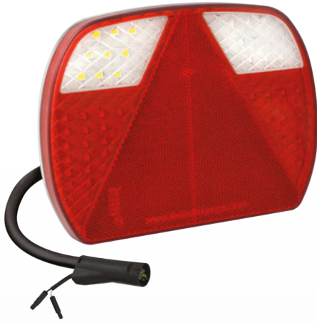
EU200 Slim-line Trailer Lamp w/ Triangle Reflector Stop / Tail / Indicator / Reverse / Fog / Reflector – 12/24V Dimensions: 195 x 148 x 22mm
