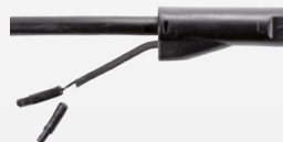
3. 6-pin rear lamp cable and connector, with integrated twin-core marker harness connection
